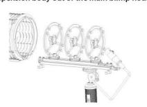
4. Loosen the locking knobs to adjust position of shockproof rings
