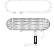
2) Straighten the fur windshield, than tighten and lock the drawstring
